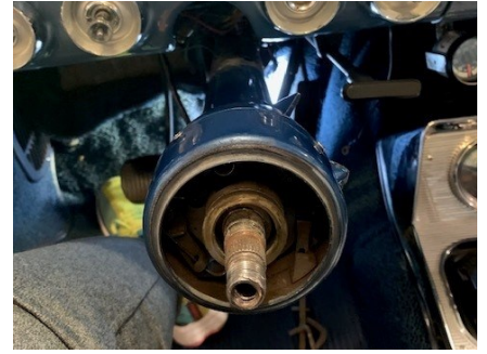
View of shaft after wheel has been pulled and column lowered by removing U shaped retainer, bolted to dash. White ring is horn contact.
