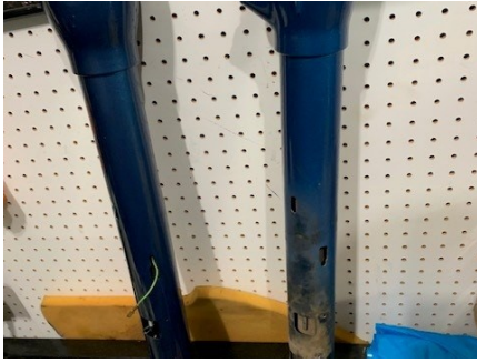
Newly painted parts car column left, old column right. Note the different openings, as left was a console shift and right column shift. Wire is horn.
