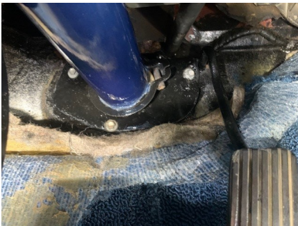
Bottom of column as installed. Used opportunity to POR 15 paint and retains to floor with 5 sheet metal screws
