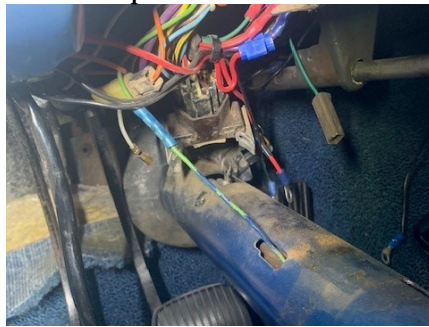
Take pictures! Column completely lowered, green wire is horn, plug is turn signals, among other grounds.
