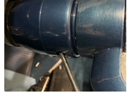
Trouble point—wheel wouldn't go 'bottom out' on splines, and gap means adjusting column up with bottom retainer to fit snug.
