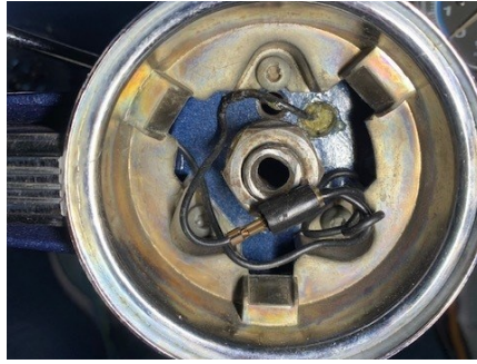
Steering wheel on, what most early 60's GM cars look like. Wires are horn connect to wheel, nut pulls wheel on splines to column shaft.
