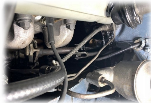
Bottom of column as installed. Used opportunity to POR 15 paint and retains to floor with 5 sheet metal screws
