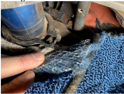
Near floorboard is adjustable column retainer w/ allen nut. Column "floats" to fit steering wheel housing.
